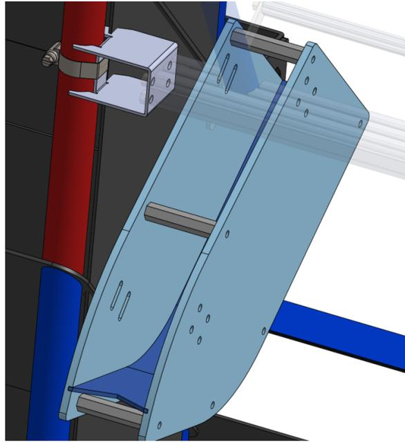
The new return rack has been completely redesigned. The outside plates are made of  $\frac{1}{4}$ " thick Polycarbonate plates, attached with zip ties to the *Tower*. The bottom plate is made of bent  $\frac{1}{8}$ " polycarbonate. AndyMark  $\frac{1}{2}$ " Churro is used to separate the two plates, with a 2" length. There is a triangular slot at the bottom of the ramp to allow *Rings* to enter the field more randomly.
